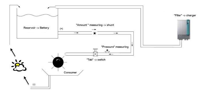
In a reservoir, a certain amount of water can be stored (**capacity**). This is conducted through a pipe to a consumer (**water wheel**).
